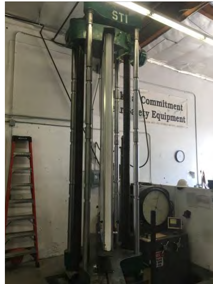
Photo 2: Axial Compression Set Up
