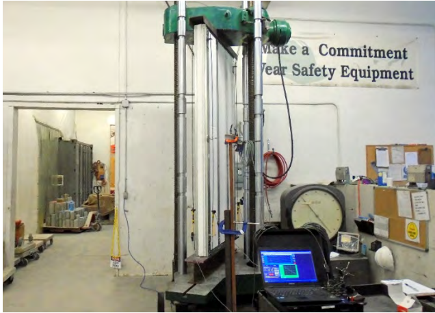
Photo 1: Axial Compression Load Test Set Up
