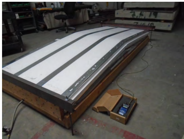
Photo 6: Typical Failure, Transverse Load Test
