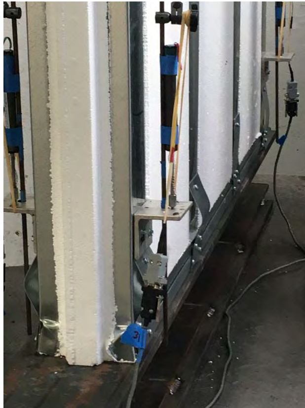
Photo 5: Typical Failure, Axial Load Test
